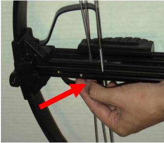
Open the magazine window by sliding the window stick forward , add up to 26 pellets.
